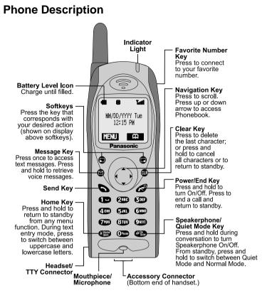
You can enter up to 32 characters by pressing the number keys. The keypad is also used to enter text as described in *Chapter 4*, "Text Entry Operations".
